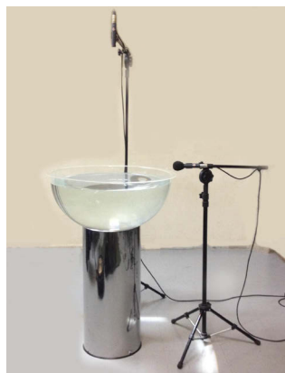
Fig.2: Microphones position and acrylic bowl.
